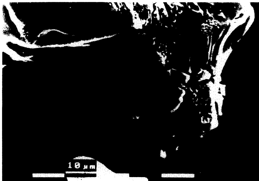
Fig. 6. Chemical attack of carbon particles during the chlorination of a \text{TiO}_2\text{-C} mixture at 910 K.
